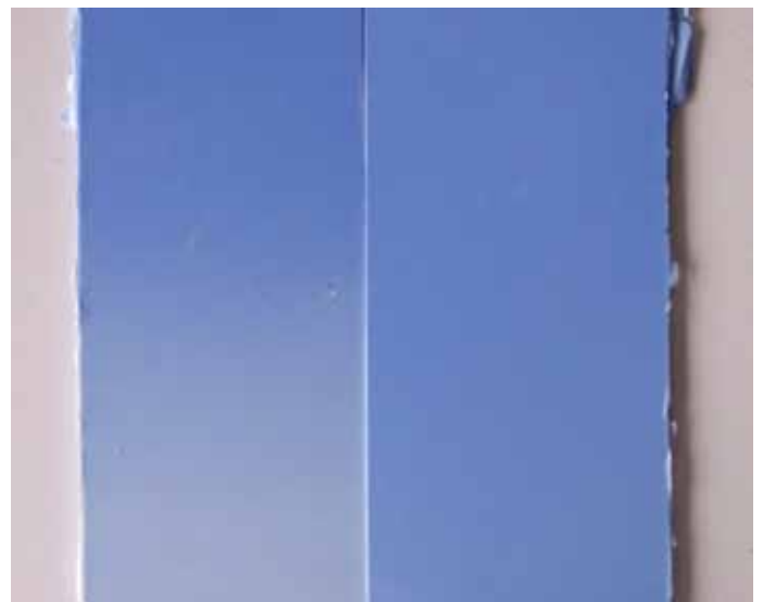
Figure 2:- Incorporated into plastic plaques, and half immersed in 20% HCl for 72 hours, Holliday Pigments' Premier XAR (right) showed 20% fading compared to the 70% fading of standard treated grades.
